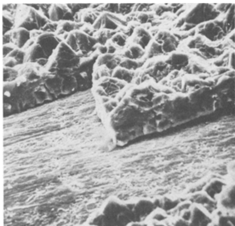
Figure 7 Scanning electron micrograph of slowly cooled, oxide scale on iron indicating top surface layer of magnetite crystallites ( \times 2100 ).
